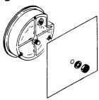
Locate mounting hole. Use double ended 1/8" thread stud. Part No. 360-f, securely inserted in center low pressure opening. Mount through a bulkhead with washer and jam nuts as in sketch. As an alternate, mount the gage
