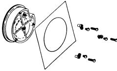
Provide a 4½" dia. opening in panel. Insert gage and secure in place with No. 6-32 machine screws of appropriate length, with adaptors, Part No. 360c, firmly secured in place. To mount gage on 1¼"-2" pipe, order optional A-610 pipe mounting kit.
